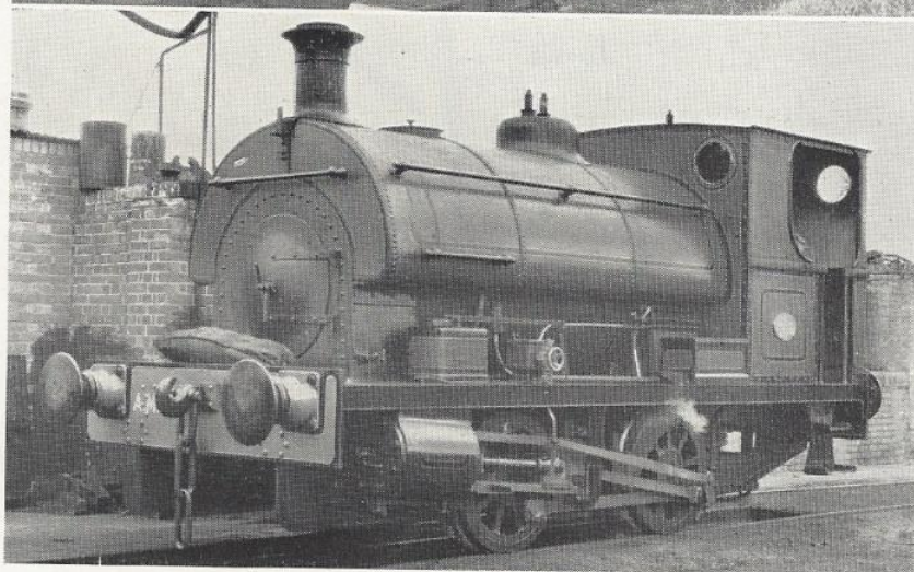
A.M.W.D. No. 127, Peckett 0-4-0 saddle tank at Cranwell, May 1953. A sack of coal is carried on the buffer beam in case the limited bunker space is insufficient on any journey
