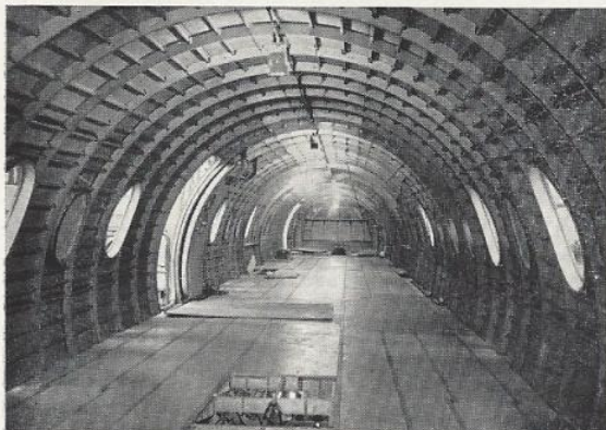
Interior views of Britannia fuselage. Left: Looking forward to the pressure dome incorporating windscreen. The large ellipse ports are escape hatches. Right: The rear portion of the fuselage showing pressure diaphragm, close stringer formation and seat anchorage rails embodied in floor gridwork
