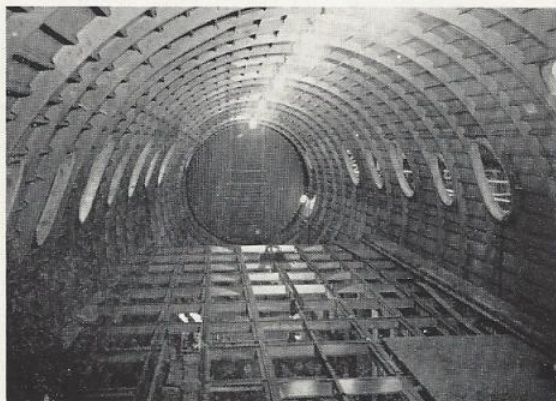
Interior views of Britannia fuselage. Left: Looking forward to the pressure dome incorporating windscreen. The large ellipse ports are escape hatches. Right: The rear portion of the fuselage showing pressure diaphragm, close stringer formation and seat anchorage rails embodied in floor gridwork
