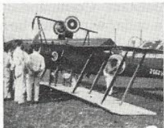
Result of a cross-wind landing
